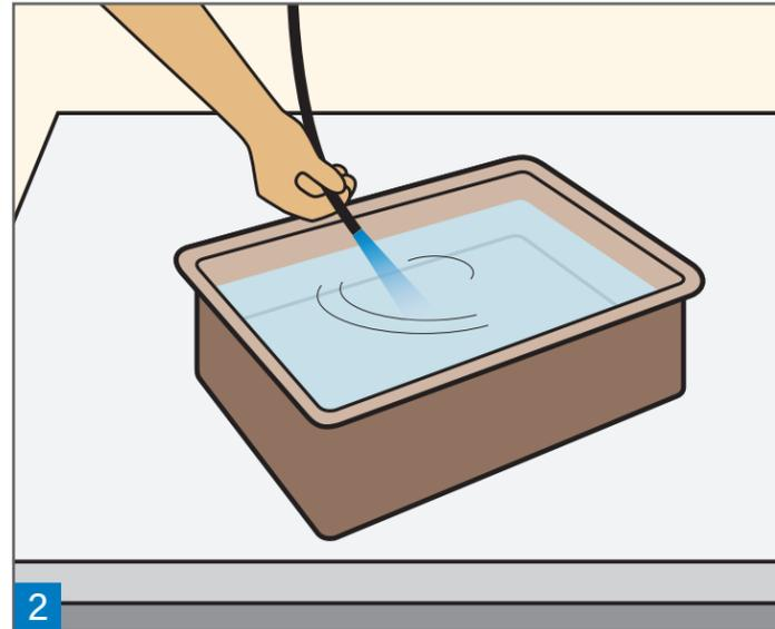
**2** Fill the tub with warm water (110 - 120° F) and allow tablet to dissolve.
